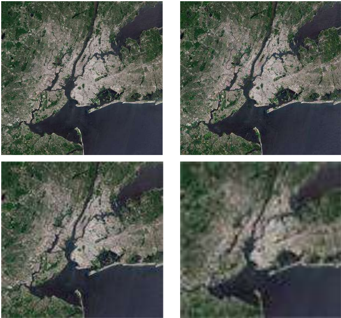
Figure.31 variations in an image's pixel resolution.
