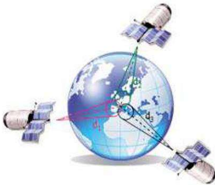
Figure 21 Triangulation principle for positioning the receiver on the ground
